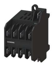
Power relay, AC-3 8.4 A, 4 kW / 400 V 3 NO+1 NC, 24 V AC, 45...450 Hz 3 pole, flat connector terminal 6.3 x 0.8mm
